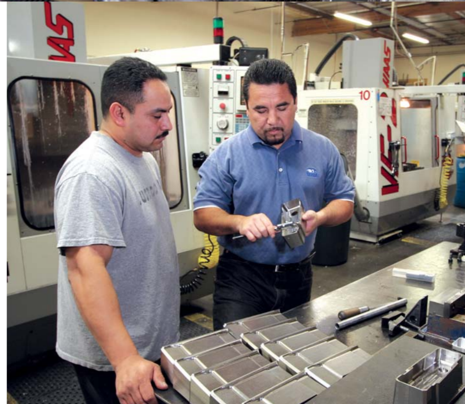
(Above Left) These thin-walled structural fittings for the F-22A fighter are machined from titanium in two ops on Mikana’s Haas VMCs. Pictured from left are op 1, op 2 and the raw titanium billet.
