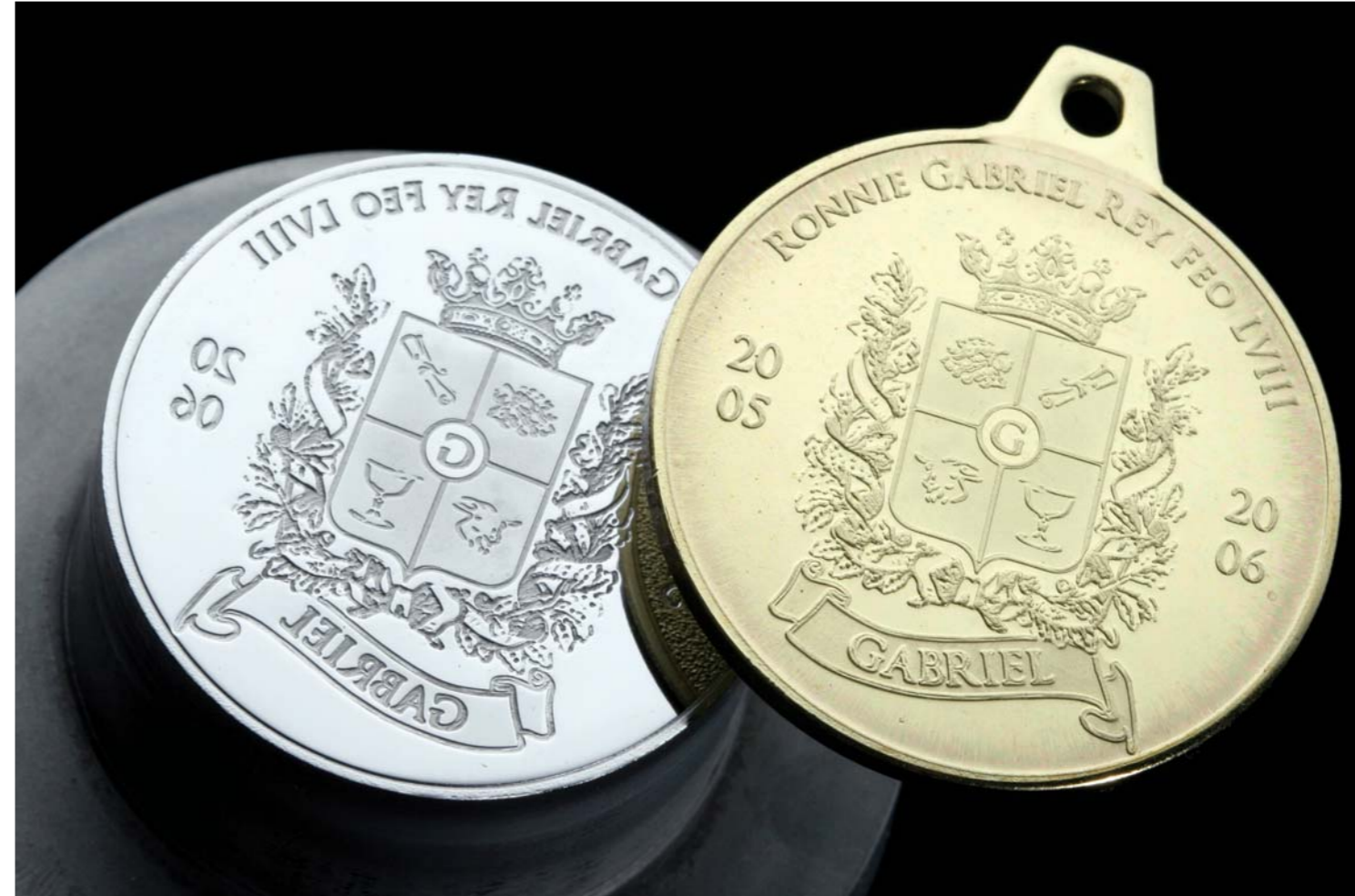
The coining die above (shown with the finished product) was designed and programmed using MasterCAM Art software (right), and machined on a Haas OM-1 Office Mill (facing page).
